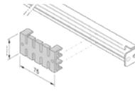
Cable retention rail for C-rail
