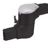
Syspend 180-Max Intermediate Joint joins two horizontal tubes together for a longer length. The arm can be rotated 300 degrees. Includes safety stop and maintenance-free bearings. Use of the intermediate joint reduces the system load rating capacity to 146 lb. (66 kg) at 3.3 ft. (1 m).
