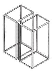
Gasket material for contained racks. To seal open gaps and minimize air recirculation.
