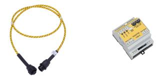
This leak detection package extends the Varistar LHX+ 45 In-Rack and the RackChiller In-Row 45 with the capability to detect leaks within the device. The rope sensor is installed at the rim of the condensate tray to minimize false alarms through condensate water or similar.
