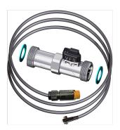
The stainless steel pipe inserts with ID 1" each come with a pair of ratiometric liquid coolant sensors. The sensors connect directly to the RackChiller Rear Door Controller. This enables monitoring of the coolant thermal properties and cooling. performance, as well as additional temperature control features.
