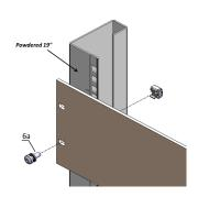
For standard grounding use a grounding nut and washer on at least one attachment point.
