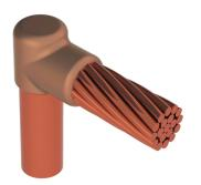
nVent ERICO Cadweld Cathodic Connections are the preferred method of exothermically welding cathodic protection anode leads to pipes (steel or cast iron), tanks, and other structures. Cathodic protection systems are designed to prevent galvanic corrosion along a pipeline or in various structures. nVent ERICO Cadweld Cathodic Connections use a special welding material alloy to minimize heat effect on the steel, which is especially important on thin wall and high stress pipes.
