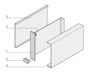
The panels protect the solder or the component side of a PCB. A coding with a separate coding strip is not possible.
