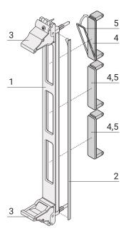
The FMC bezel are in accordance with Vita 57.1 specification. Covers the cut out in the overall front panel.
