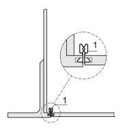
For vertical stainless steel EMC shielding between recessed mounted shielded front panels and side panel.
