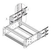
Adapter for rear fixing of a subrack in accordance with DL3 standard into a cabinet. It guarantees shock and vibration resitance up to 25 g.
