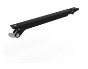
The HF311 Series was designed in accordance with VITA 48.4 and 48.5 to provide up to 20:1 mechanical advantage for insertion and extraction of printed circuit boards with high density connector contacts. The integrated spring provides positive pressure on connectors during Card Lok actuation and consistent self-compensation for board tolerances. The HF311-TC is ideal for 2nd level maintenance; can be operated with a gloved hand and no specialized tools are required.
