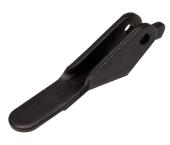
The Series 71 provides extraction assistance of printed circuit boards with high density connector contact and multiple connector applications. With a 4.5 : 1 mechanical advantage, the Series 71 can be used for cold wall applications with any SCHROFF Card or Wedge Loks, or with sheet metal enclosures when using the Series 24 or 127 PCB Tainers with the optional flange feature.
