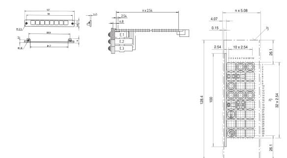
Mounting frame for mounting plane 1, Flammability UL 94 V0 and two threaded female connectros M2.5.
