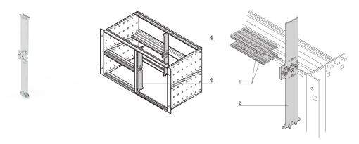
The support is bolted into the grid holes of the horizontal rails and allows a split of a 6 U subrack in 2 x 3 U parts.
