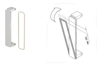
The O-ring gasket can be used for EMC shielding of PMC or FMC mezzanines. The O-ring will be assembled into the groove of the Mezzanine.
