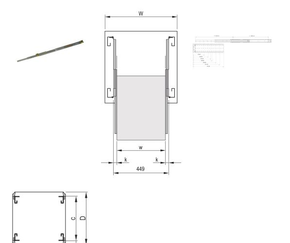
Narrow Telescopic Slide for Subracks with > 100 % extension.
