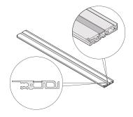
The cover strip can be inserted into a groove on the rugged horizontal rail and covers the perforation of the horizontal rail for fixing the guide rails.
