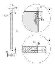
Flat front panel. Shieldable with stainless steel EMC gasket.
