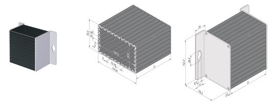
The rectangular Alu-profile case enables a user to insert 4 standard PCBs (height 100 mm x depth 160 mm). The PCBs will be inserted in grooves in the Alu-profile tube. Both sides are covered with 2.5 mm thick L-shaped front panels for wall mounting.
