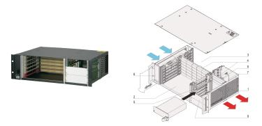
3 U CompactPCI System with horizontal Card Cage for six 6 U Boards, six RTM Boards and one CompactPCI 3 U Pluggable Power Supply. Option to assemble up to three pluggable Power Supplies.
