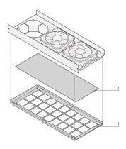
The air filter filters the intake air and reduces the quantity of dust or other particles.
