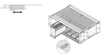
Additional securing of the rugged cover plate to protect against shock and vibration. The Kit will be screwed onto the top / bottom cover. A movable bolt engages under the horizontal rails and thus provides additional fixing.
