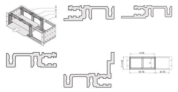
Board cage for horizontal boards offers the option to insert 6 U boards in a 3 or 4 U high subracks or desktop cases. Pease add a front front panel to cover the assembly Kit.
