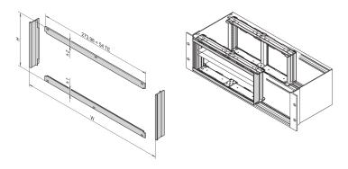
Front frame installation provides the contact between subracks and assemblies. It must be used if a customer has selected a horizontal board mounting Kit.
