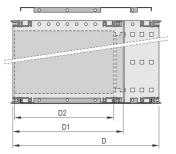
EMC Shielded subrack for backplane mounting, for CPCI application.
