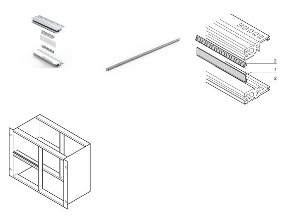
The contact strip makes contact bewteen horizontal rails. If two horizontal rails are mounted one above the other, the seals plus a metal strip enable EMC shielding.
