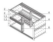
The combined mounting enable the option to split a 6 U high subrack or case in 2 x 3 U and 6 U sections. Different versions are available.
