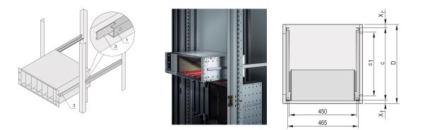
The C-profile, assembled on the Side Panel of the subrack serves fixes the subrack on the guiding profile when mounted into a cabinet.
