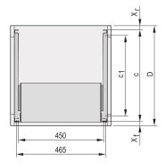
The C-profile, assembled on the Side Panel of the subrack serves fixes the subrack on the guiding profile when mounted into a cabinet.
