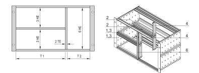
The combined mounting enable the option to split a 6 U high subrack or case in 2 x 3 U and 6 U sections. Different versions are available.
