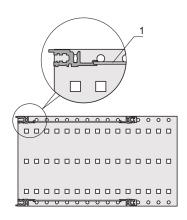
Mechanical covering of installed components. The plate is inserted into a groove of the L type horizontal rails.
