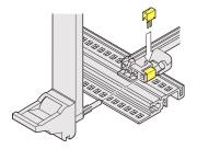
ESD clip can be plugged into the keying/coding block of the guide rail with coding. Provides an conductive contact between the alignment pin of the inserter/extractor handle (IEL or IET) and the horizontal rail.
