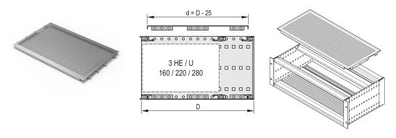
A cover plate is used for electromagnetic shielding or as mechanical protection. The cover can be screwed onto the side panel.
