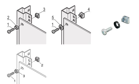
For standard grounding use a grounding nut and washer on at least one attachment point.
