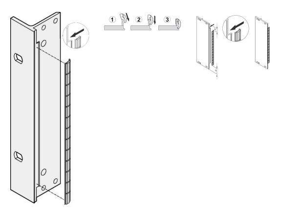
The stainless EMC gaskets are inserted into a slot on the right hand side of the U-shaped front panels.
