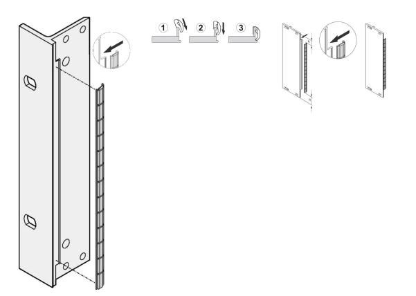
The stainless EMC gaskets are inserted into a slot on the right hand side of the U-shaped front panels.
