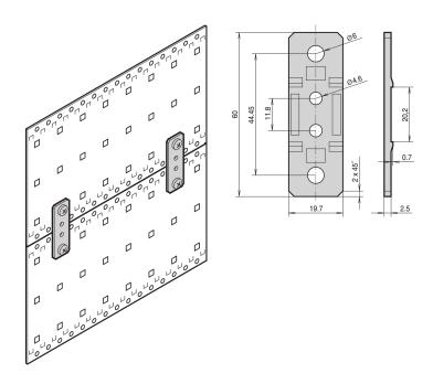
The brackets are used to connect the fan units to the side panels of a subrack.
