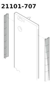
The stainless steel EMC gaskets are inserted into the lateral slots of the shieldable front panels (2 pieces per front panel).
