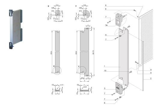
Plug-in unit, with IET inserter/extractor black handle, 3 U, front assembly. The U-shaped front panel enable shielding with a textile gasket.
