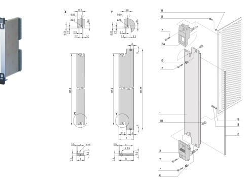
Plug-in unit, with IET inserter/extractor black handle, 3 U, front assembly. The U-shaped front panel enable shielding with a textile gasket.
