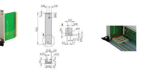
Plug-in unit, with IEL inserter/extractor black handle, 3 U, rear I / O assembly. The U-shaped front panel enable shielding with a textile gasket.
