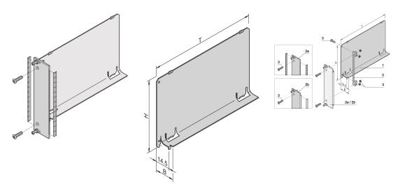
The air baffle with flat front panel covers an empty slot and eliminates an air leak. The flat front panel accepts a stainless steel EMC gasket.
