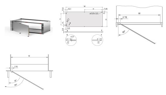
Front panel with textile EMC gasket, side hinged assembly.
