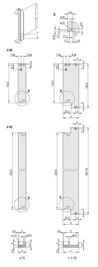
Plug-in unit, with IEL inserter/extractor black handle, 6 U, front assembly. The U-shaped front panel enable shielding with a textile gasket.
