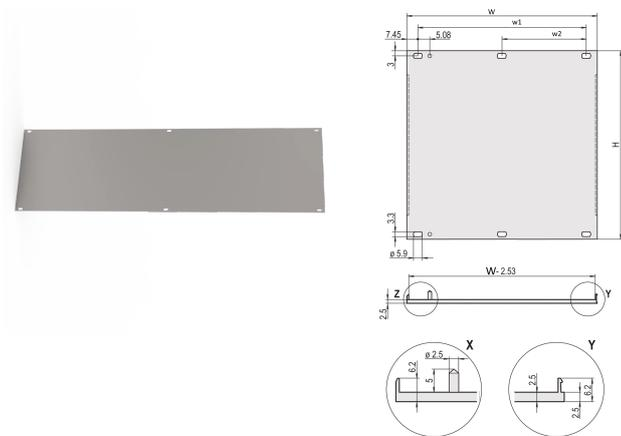
U-profile front panel for textile EMC gasket.
