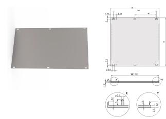
U-profile front panel for textile EMC gasket.
