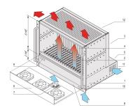
VME64 system for 21 VME64x boards 6 U, 160 mm. Rear I/O option The power for the system is supplied by a open frame power supply. A fan control module monitors the fans, the temperature and voltage.
