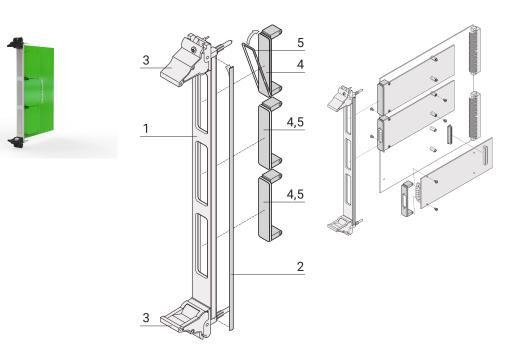
The FMC bezel are in accordance with Vita 57.1 specification. Covers the cut out in the overall front panel.
