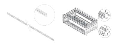
The threaded insert is a metal strip with thread M2.5 and allows the fixing of front panels.
